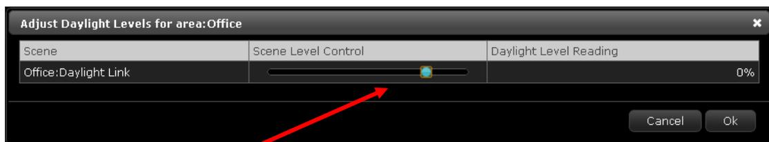
Adjust the level using the slider until your lux meter reads the level that you want (perhaps 500 lux at desk level?). The slider will proportionally adjust the levels of all channels in the scene.
