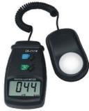
You will require a light level meter in order to commission the light level set-point for your daylight harvesting / constant-light level control. Place the light meter's sensor at the position where you want to measure your set-point, for example on the desk surface.
